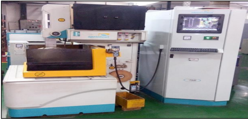
Wire cut Machine for Die Manufacturing Make – Electronica (India) BED SIZE- 300x400x200 (Accuracy :- 10 Micron)
