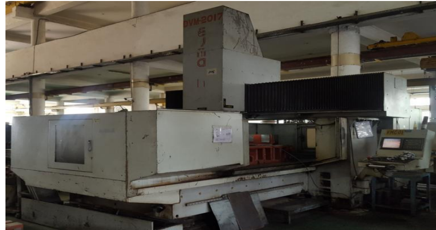
Double Column VMC, Make - Eumac BED SIZE- 2200 X 1600 X 700 MM
