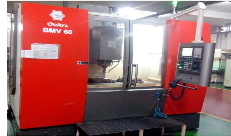
3 Axis VMC for Die Manufacturing, Make – BFW , BED SIZE- 1250x600x630 (Accuracy :- 50 Micron)
