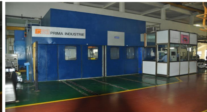
5 Axis Laser Cut, Make – Prima (Italy) BED SIZE-4000x2500x1000 (Accuracy 50 Micron)
