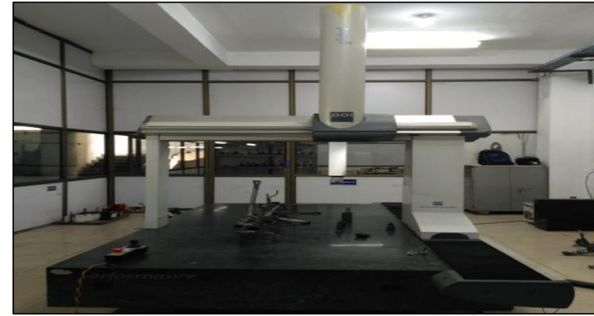
CMM, Make- Brown & Sharp, (USA) Bed Size- 2200 X 1200 X 1000 MM Accuracy :- 01 Micron
