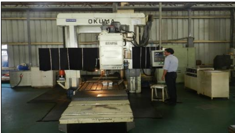
CNC Jig Boring Machine for Die Manufacturing Make – Okuma (Japan) BED SIZE- 1800x1000x1000 (Accuracy :- 20 Micron)
