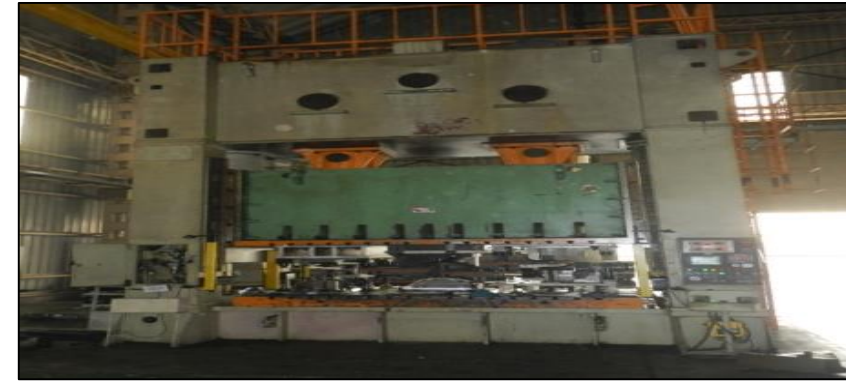
Tool Trial Press Make- Yangli (China) 400 Ton HIGHLY PRECISED
