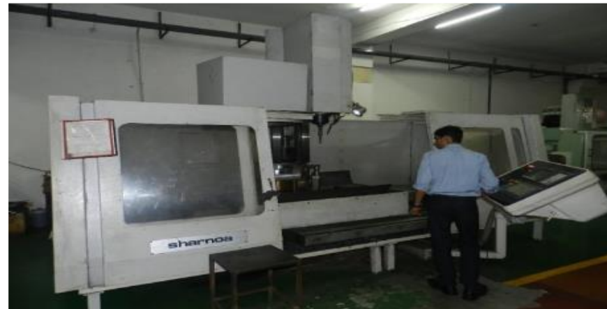
3 Axis VMC for Die Manufacturing, Make – Sharnoa (Swiss) BED SIZE- 1400x700x650 (Accuracy :- 50 Micron)
