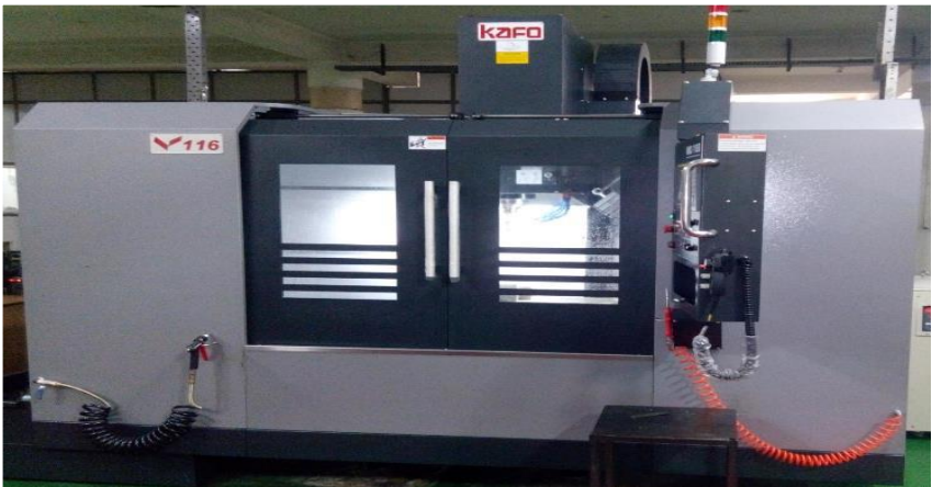
VMC Machine, Make – Kafo (Taiwan) BED SIZE- 1100 X 600 X 600 MM (Accuracy :- 30 Micron)
