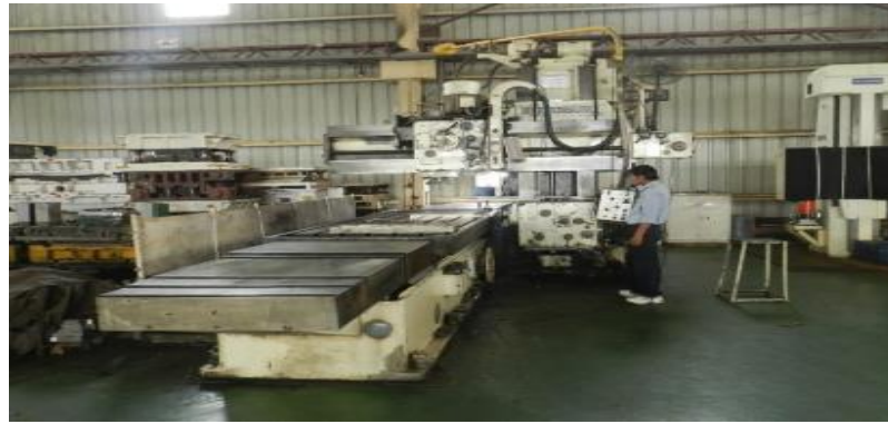
Plano Millar for Die Manufacturing Make – Kotobuki (Japan) BED SIZE- 3000x1100x800 (Accuracy :- 50 Micron)
