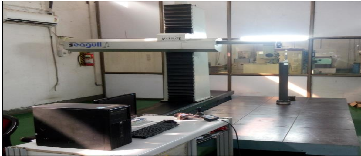
CMM : 01 No's Make – Accurate (China) Bed Size – 3000 x 1600 x 1600 mm, Accuracy :- 01 Micron
