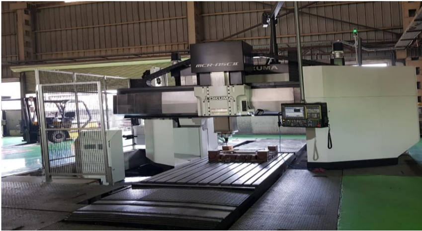
VMC 5 Axis, Make – OKUMA, BED SIZE- 2000 X 3000
