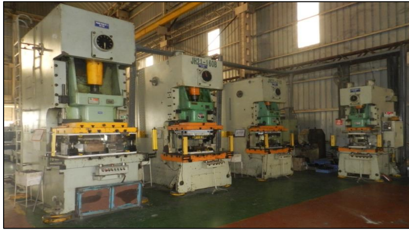
Tool Trial Press Make- Yangli (China) 63 Ton to 250 Ton HIGHLY PRECISED
