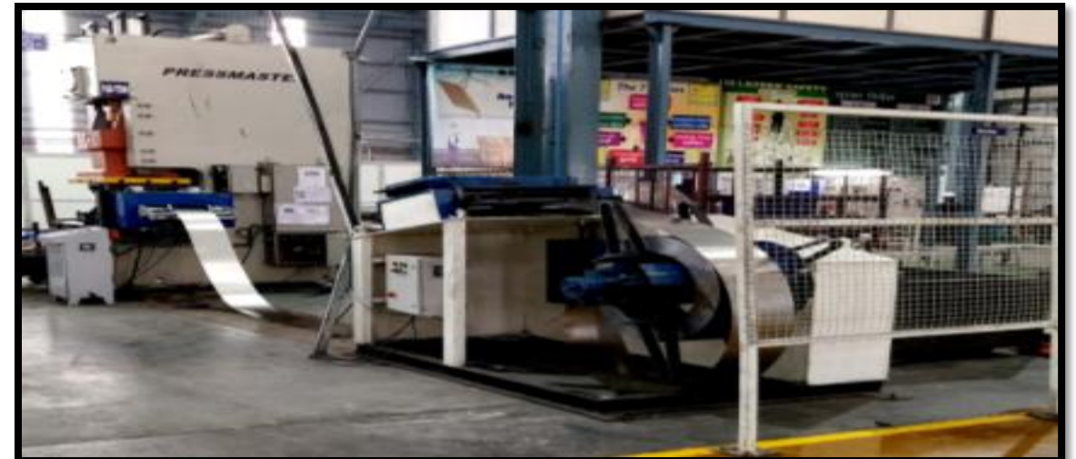
2 COIL FEEDER (200 TON + 160 TON)
